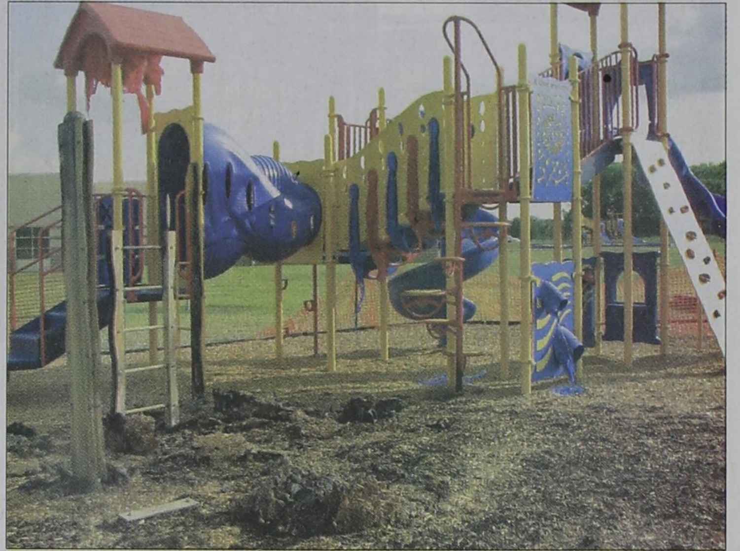
A large charred spot is seen after some of the damage was cleared away following a fire that destroyed part of the play equipment at Miss May Vernon Elementary School in Fate. Illegal fireworks are believed to be the culprit, first igniting the wood chips at the base of the play set then quickly spreading to the plastic equipment. Some melting can be seen on the underside of the red cover at left, on the red and blue supports at center and to the blue tubes on the right. Photo by Kathy Williams/Rockwall County News
