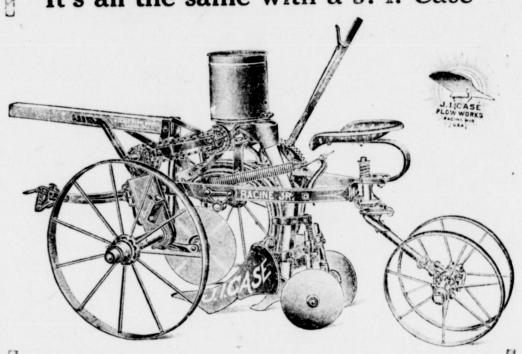
We want to show one thing about this Lister. A slotted curve casting controls the movement of the beam. The point of the middlebuster always travles up or down faster than the heel, consequently penetration is secured at any height.
