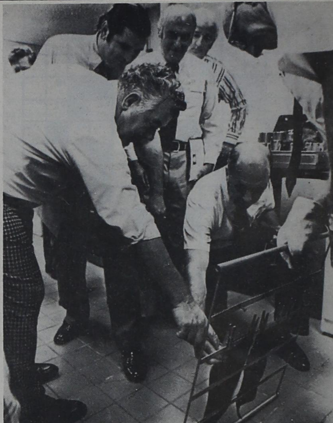
FIREFIGHTERS MEASURE CHAR —Members of a fact finding delegation from the New York City fire department take a close look at char lengths on fabric samples at the Cotton Incorporated Research Center at Raleigh, N.C. Kneeling (right, knee on floor) is Chief John R. Travell of the New York City fire department division of safety. Leaning over (left) is Lt. Thomas Montgomery of the Uniformed Fire Officers Association. After him are (left to right) Dominick Gentiluomo, Sergeant at Arms for the Uniformed Firefighters Association; Pete Avery, chief's aide; and Jim Hangle, Cotton Incorporated director of apparel mill marketing. Holding the rack (wearing glove) is Dr. Leonard Smith, Cotton Incorporated associate director for fire retardance research.
