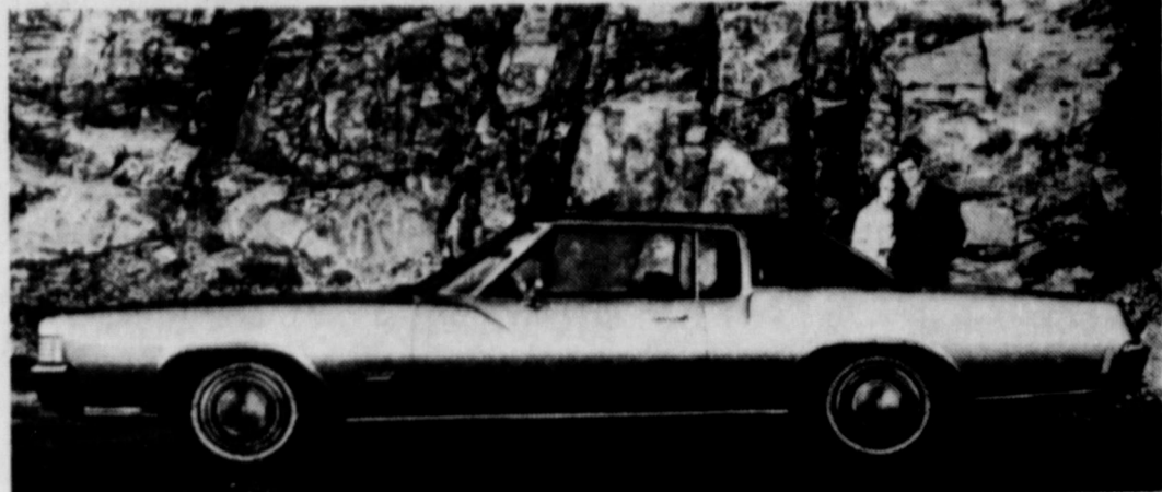
For 1971, the wheelbase on Oldsmobile's front-drive Toronado is 122 inches, three inches longer than previous models. Displaying a unique and unmistakable elegance, the Toronado is also a
