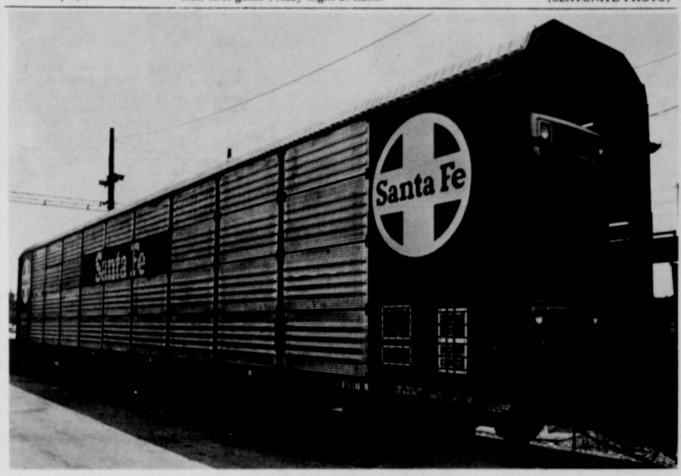
NEW DESIGN —First of its kind in the railroad industry, new Santa Fe bi-level rail car is designed to carry 12 trucks in a protected environment from factory to dealer.
