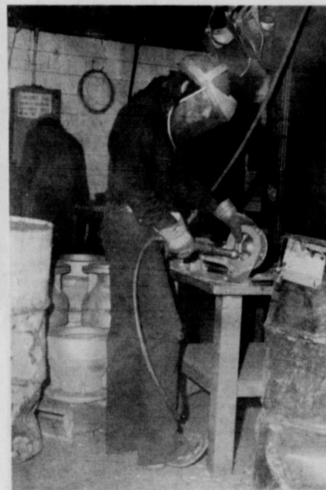
LAST STEP — Grinding away the rough edges is the final step before castings are ready for shipping. Peter Cantu is using a high speed grinder to smooth grooves of a casting.
