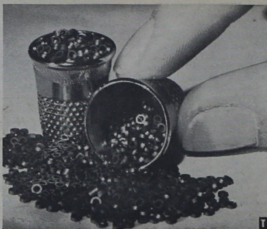
These tiny doughnut-like cores, the electro-magnetic building blocks for many modern computer memories, are made by IBM in almost microscopic sizes. A typical computer memory might contain more than a million such cores. Each is separately tested during production.
