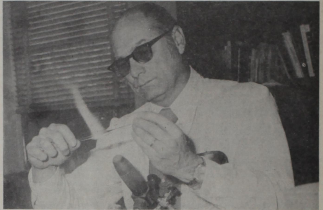
CREATING AN ORNAMENT—Victor Johnson, glass working shop supervisor in the chemistry department at Texas Tech University, often uses his glass blowing skills to create unusual Christmas ornaments. After heating the glass, Johnson blows it into whatever shape he wants. A silvering solution is poured inside the ornament before Johnson paints its exterior. (Times Photo)
