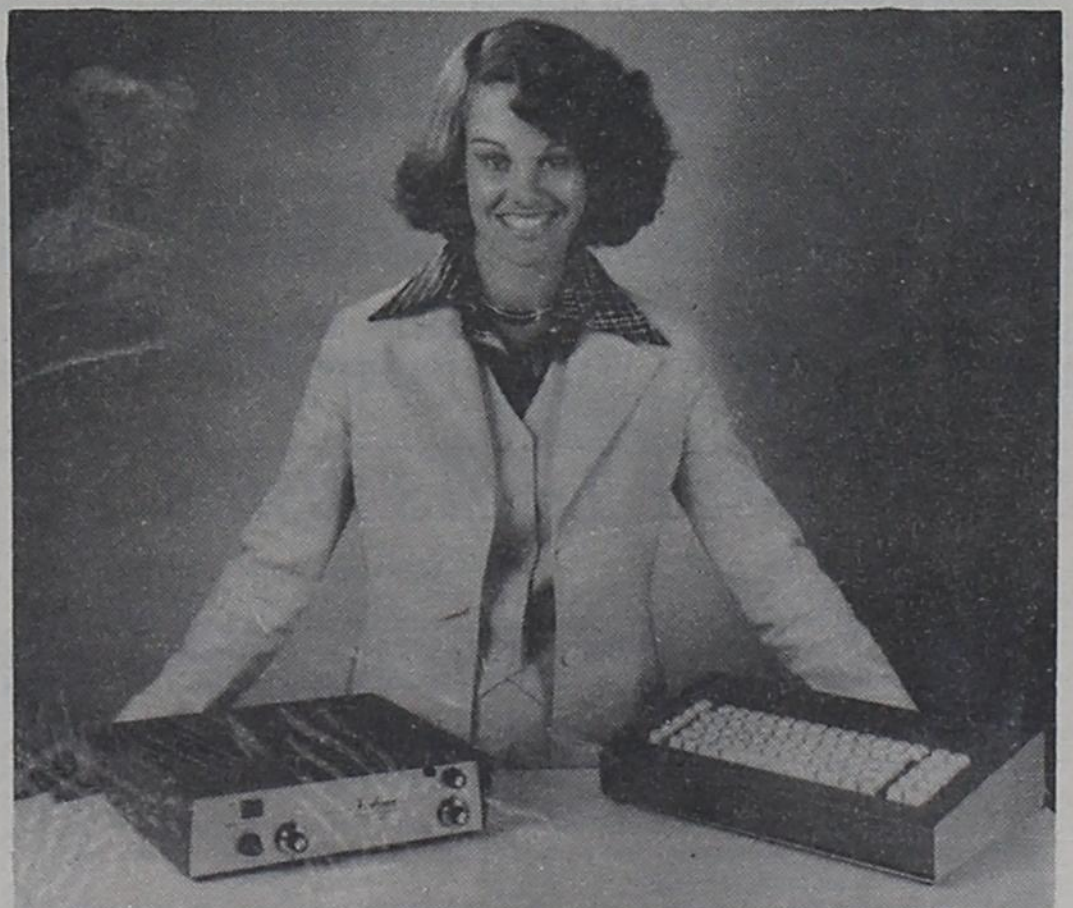
THE TALKING COMPUTER —This voice synthesizer, or talking computer, is an electronic device which produces simulated human speech through selective programming of phonetic sounds. In a unique demonstration by General Motors "Previews of Progress" lecturers, this exciting alternative to visually-oriented data processing is shown to have virtually unlimited future applications. The talking computer is one of nine dramatic experimental science demonstrations in the Previews show now appearing in this area. The 40-minute admission-free presentation by two lecturers highlights the many career opportunities available as a result of research in science and engineering.
