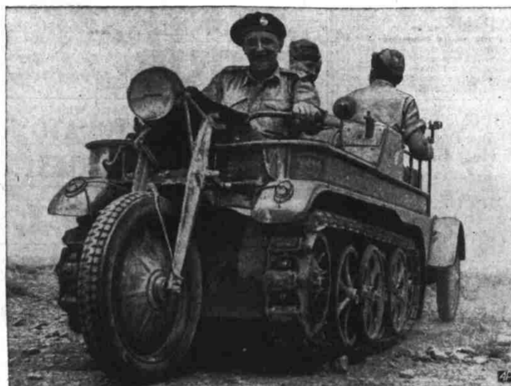
NEW AXIS VEHICLE — This new type of motor-cycle track vehicle was captured from the enemy by the British in Libya. It is used to tow small guns and carry a few men.
