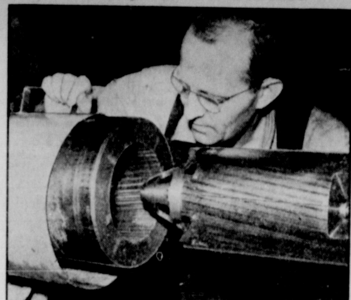
Robert Sneridan views the rifling of a 155-millimeter gun, made by the shaft at right, in the Watervliet, N. Y., arsenal, where artillery is being rushed for the national defense program.
