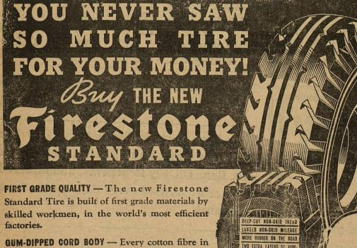
every cord in every ply is soaked in liquid rubber. preventing internal friction and heat, which provides greater strength and blowout protection.
