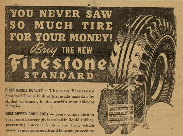
TWO EXTRA LAYERS OF GUM-DIPPED CORDS UNDER THE TREAD - This patented Firestone feature cushions road shocks, protects against punctures and gives longer life.
