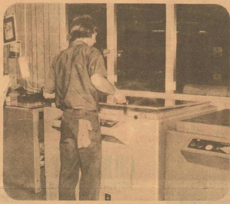
5 The negative is put on a metal plate and exposed to ultra violet light. The light creates a chemical change on the metal plate. The plate is then developed like a photographic negative. It is then ready to be put on the press.
