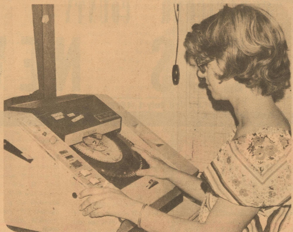
2 The salesman turns in all the large print to be set. Here Nell Edmiston sets type on the headliner. The letters will be much larger than the type you are reading. The number 2 in this box was done on the headliner.
