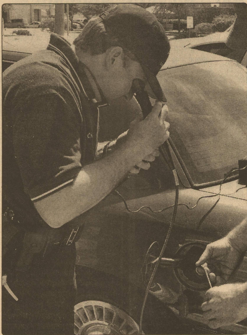
PHOTO BY KATHY MANKIN Open wide and say, Aaaah — Deputy Jason Chatham demonstrates a new scope that allows local officers to look for drugs inside fuel tanks or other hard-to-check places.
