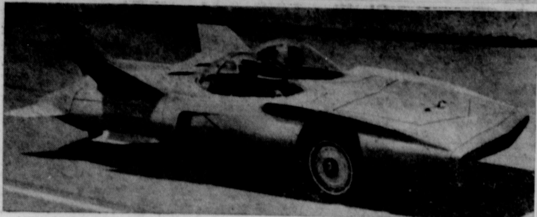
YOU CAN'T BUY ONE —Strictly experimental, this electronically controlled car goes through its paces on a California test track. Named "Firebird III," it features a single, stick-like control, much like the control of some small planes. With this device the driver steers, brakes and controls the car's speed. Gas turbine in rear drives the vehicle; a 10-h.p. conventional motor under the hood provides power for the machine's accessories.
