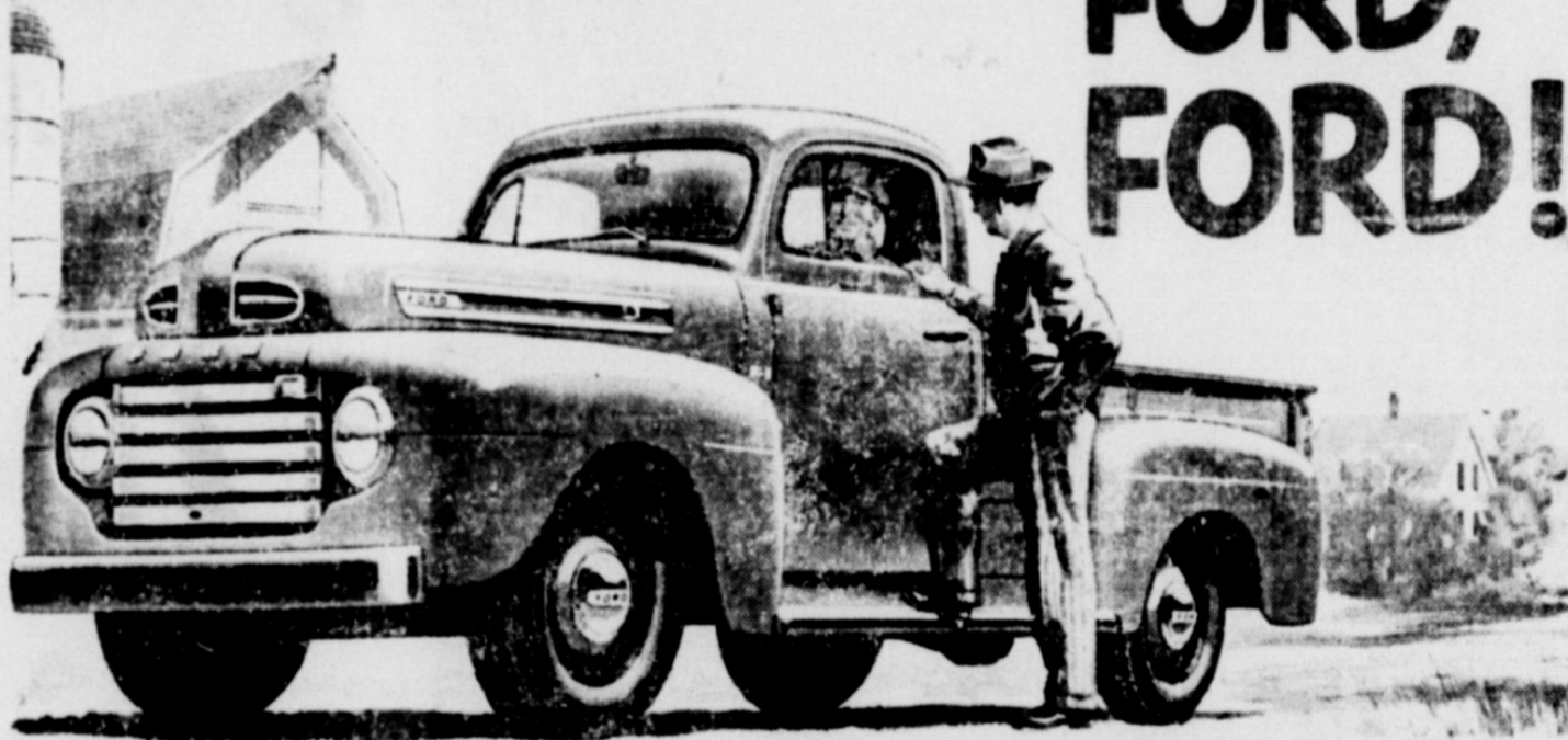
4½ ft. Ford F-1 Pickup shown here. G.V.W. rating—4,700 lbs. Body capacity—45 cu. ft. Available with 95-h.p. Six or 100-h.p. V-8. One of over 175 models including 145-h.p. Big Jobs.
