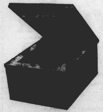
Made of heavy gauge steel inside and out, all electric welded, between these steel walls is 11/2 inches of solid Fire Proof Vermiculite Insulation which has over 300,000 tiny air cells to the square inch. It has the universally used tongue and groove principle around the door with 11/2-inch fireproof seal completely around it. Outside dimensions 14x111/2x 71/2 inches. Inside dimensions 81/2x11x 11/2 inches. Equipped with heavy standard type key lock, with two keys. Very attractive gray finish.
