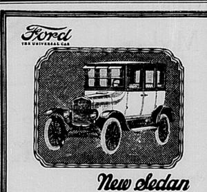
A higher radiator with a trim apron at its base lends dignity befitting a closed car. The higher hood and enlarged cowl curving gracefully to the dash give a stylish sweep to its body lines, and afford additional leg room for occupants of the front
