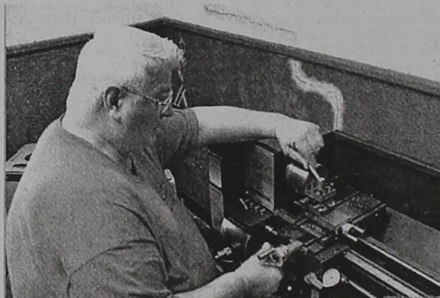
DENNIS ALLEN is working at the metal lathe to machine the zinc coated bolt that will become the sensor probe for the Lawn Angel.
