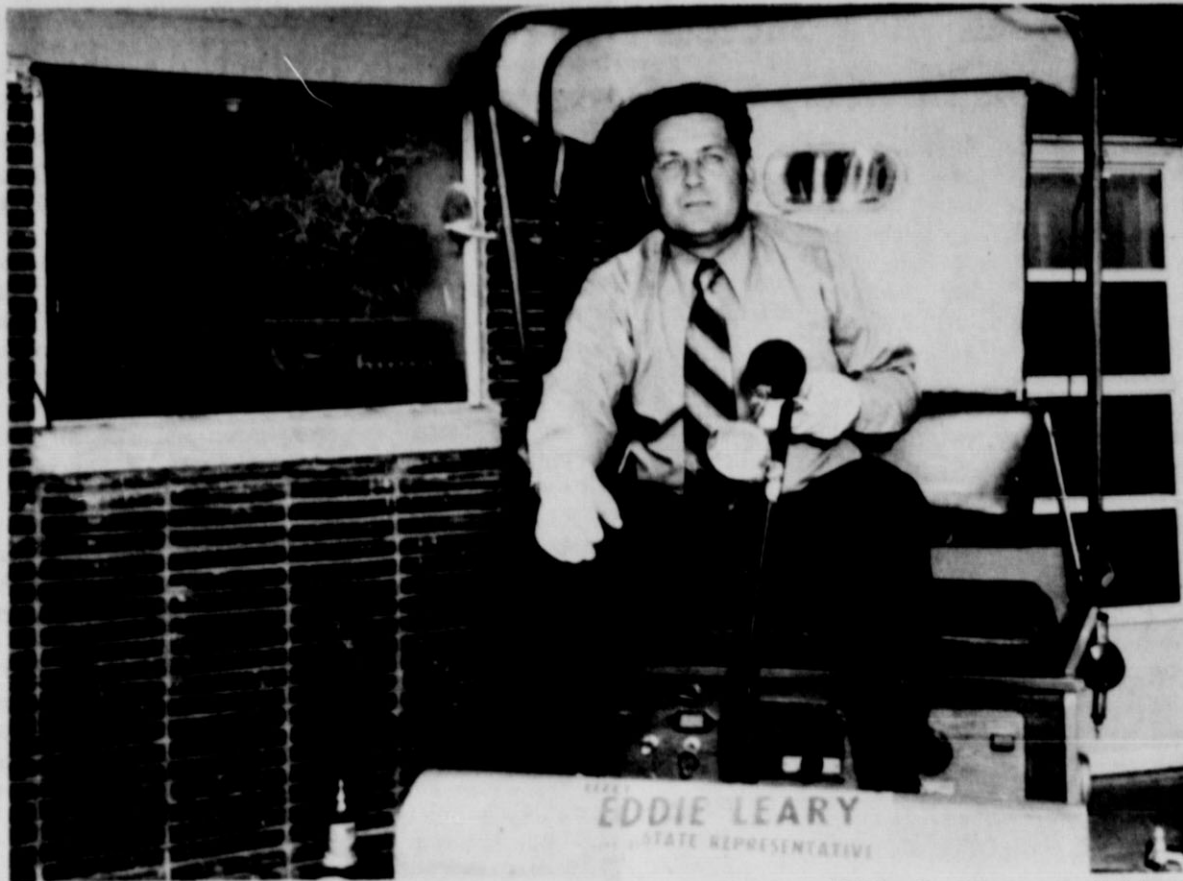
ON HIS WAY — Democratic candidate for State Representative Eddie J. Leary of Childress, native of Motley County, was here recently, driving his 7 HP (¾ size to scale) 1901 Oldsmobile. The car was made in Childress by Charles Jones, manager of the Childress Compress Co. The car has a top speed of 20 mph and the gas tank holds one gallon. Above photo was made in front of the Tribune. Leary transports the "horseless carriage" from town to town in a pickup truck.
