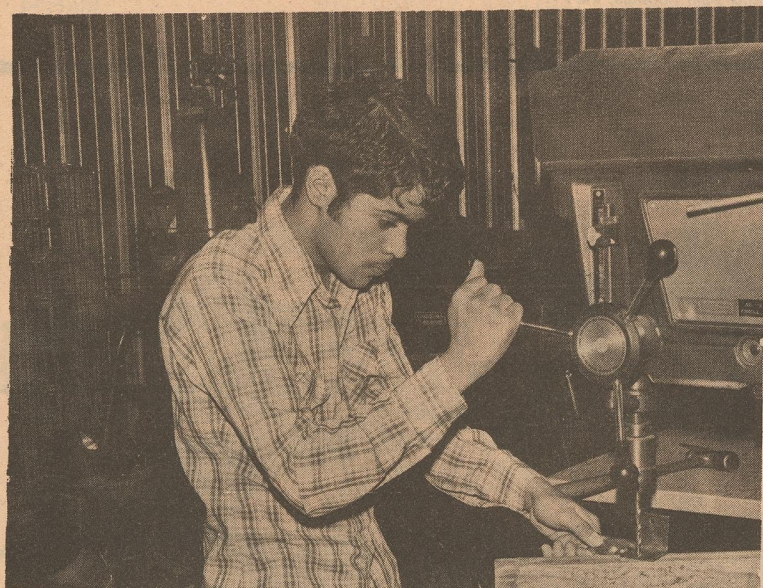
Mark Guerrero drilling for braces for bleachers.
