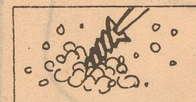
Soaping the threads makes it easier to screw a wood screw into wood.
