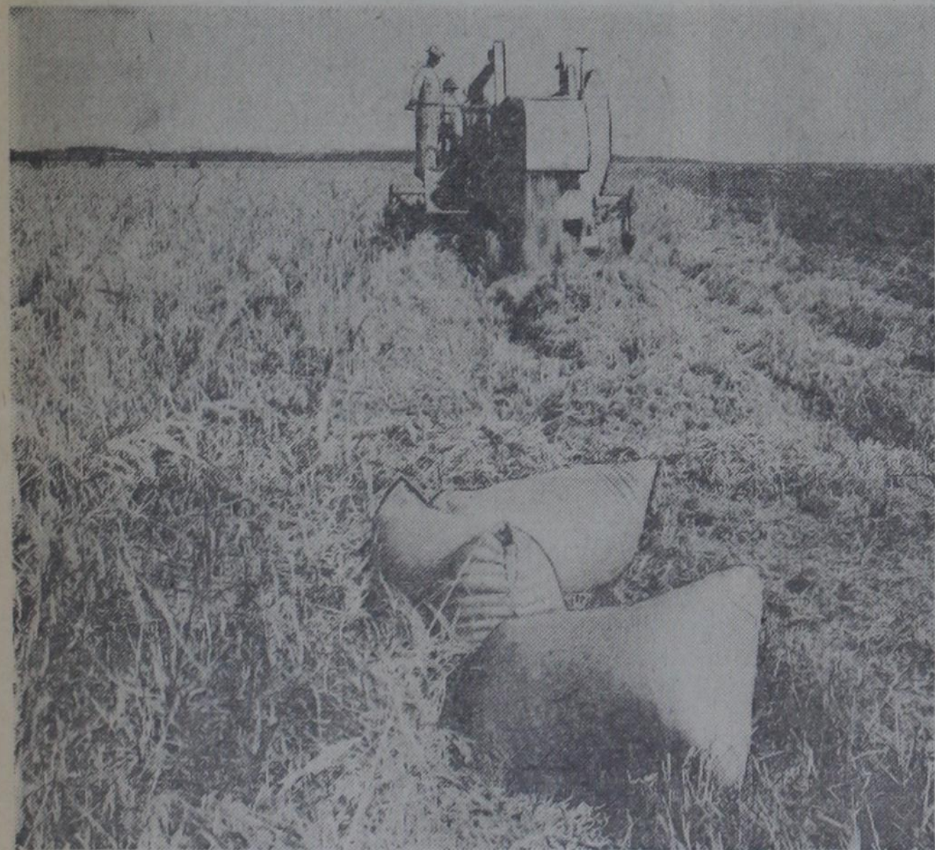
Harvesting rice in South Texas. The combine cuts, threshes and sacks the rice.
