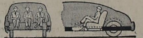
NEW HUDSON—You ride cradled down within Hudson's base frame, as shown above, and also ahead of the rear wheels. Seats can therefore extend full width of the car. Due to the use of the "step-down" zone, roof is lowered for streamlining, yet ample head room is provided.
