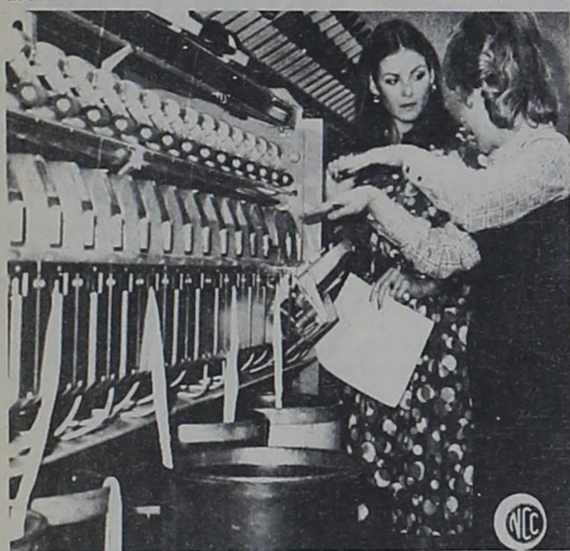
NEW SPIN FOR COTTON —Maid of Cotton Kathy Raskin gets the inside story on a new open-end spinning system from Nell Raper of Texas Tech's Textile Research Center in Lubbock. The frame, which was donated to the center by Plains Cooperative Oil Mill, promises to widen the use of short staple cottons. It spins at a much faster rate than conventional systems.
