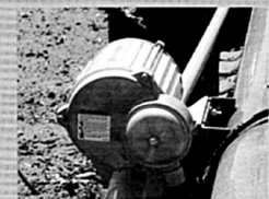
Valley, Centerdrive Conversion on a Zimmatic Planetary
