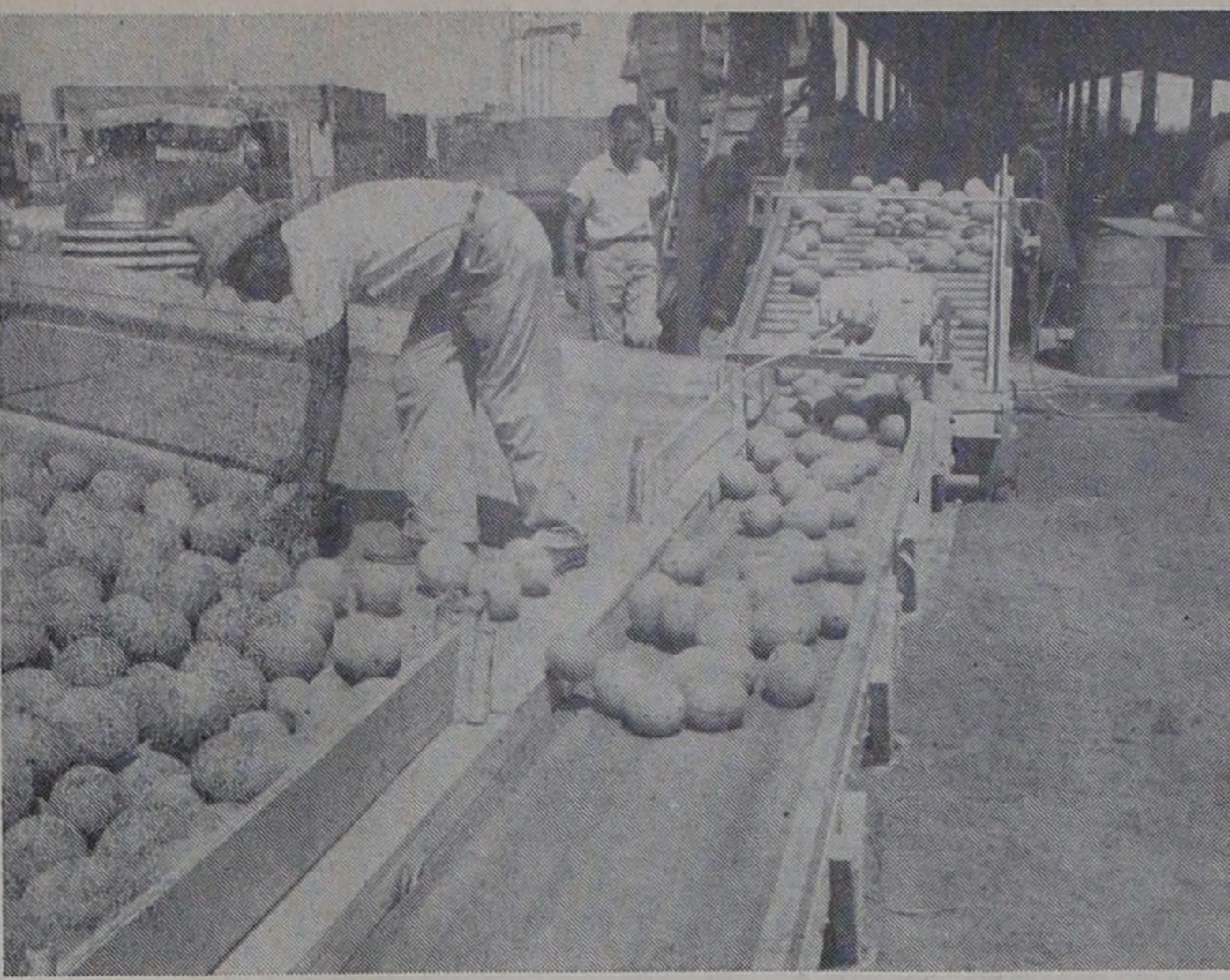
ROLLIN' 'EM IN to the Gateway Produce Company's processing operation in this shed hand who lifts small wooden gates and starts the cantaloupes gently tumbling down to meet a conveyor belt, where they are lifted into the shed. Once inside they are graded and packed by hand.
