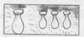
One 75 watt bulb gives more light than three 25 watt bulbs.
