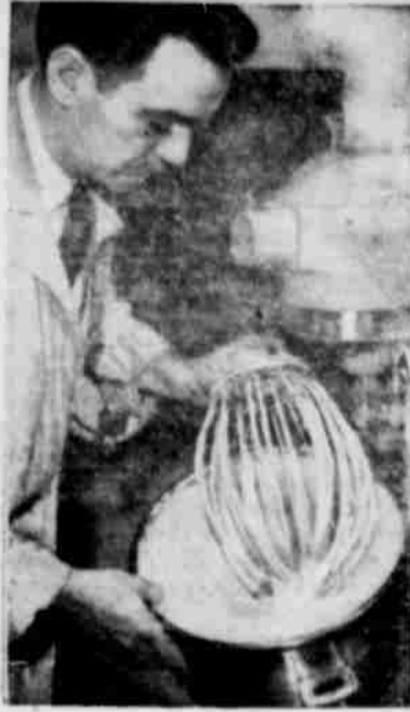
CAKE BATTER? No, it's a test bath of foam rubber being examined by chemist in pilot plant of a control laboratory.
