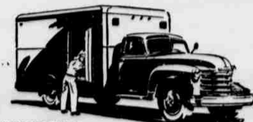
HEAVY-DUTY CAB-AND-CHASSIS with Refrigerator Body Model 6403—161-inch Wheelbase Maximum G.V.W. 16,000 lb.
