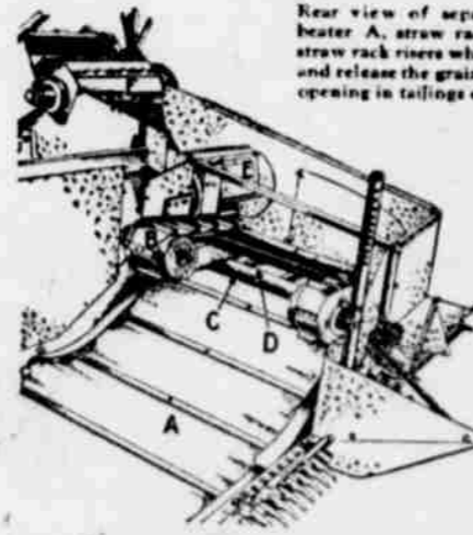
Elevator and feeder. A, platform and lower elevator canvas. B, upper elevator canvas cut away to show extra roller C, and carrier D. E, saw-toothed beater; F, spiked beater, which helps to carry grain to cylinder.
