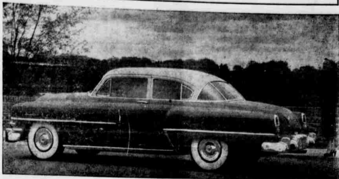
Smart new lines mark the 1953 Chrysler New Yorker club coupe. New Yorker models are offered in a choice of 6-passenger sedan, club coupe, special Newport club coupe, Town and Country wagon and 8-passenger sedan on a wheelbase of 125 1/2 inches. Powered by the Chrysler 180-horsepower FirePower V-8 engine, they feature power brakes and Oriflow shock absorbers as standard equipment. They are available with full-time power steering as optional equipment.
