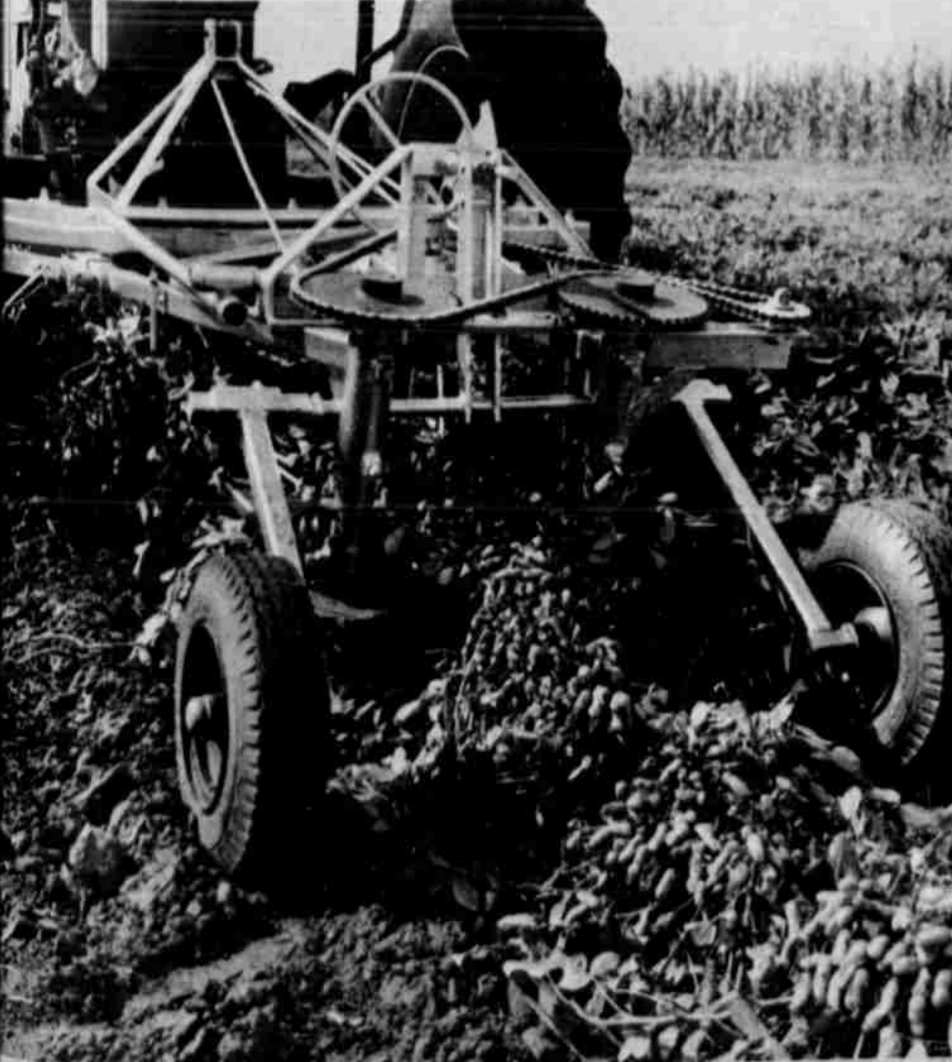
PEANUT PICKER—A close-up view of the peanut harvester illustrates how it extracts them from the ground, then turns plants on their backs so that the fruit is exposed to the sun to dry and so that it easily shed any rain that may fall. The variety of large, fancy peanuts shown here are highly suitable for the soil and growing season of Lamb County. Growers expect approximately 2,500 pounds of peanuts to the acre and a price of 15¢ per pound this year. Processing is done at Portales, N. M.
