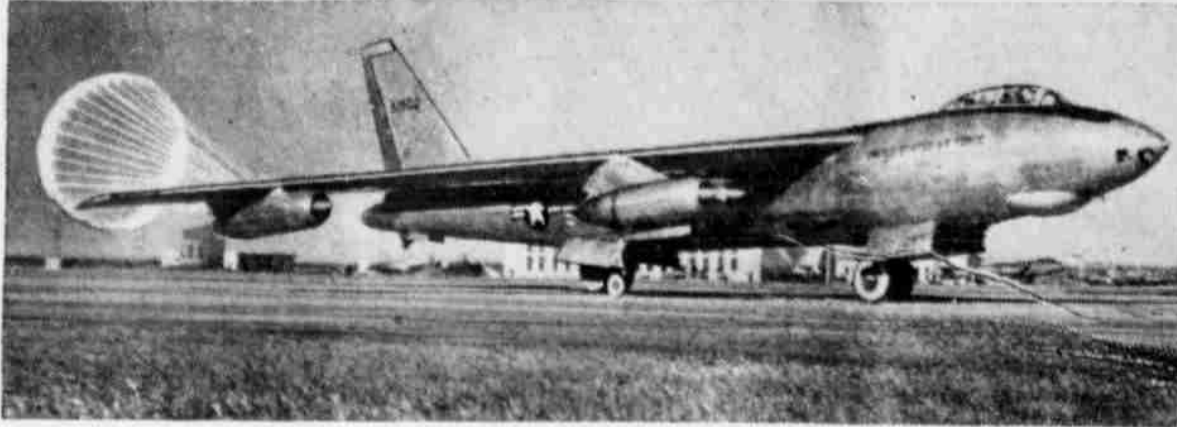
WHOA! SAYS THE PARACHUTE, decelerating this Stratofortress on a runway at Wichita, Kan. It gives a big assist to the anti-skid braking system on the tandem-type landing gear.
