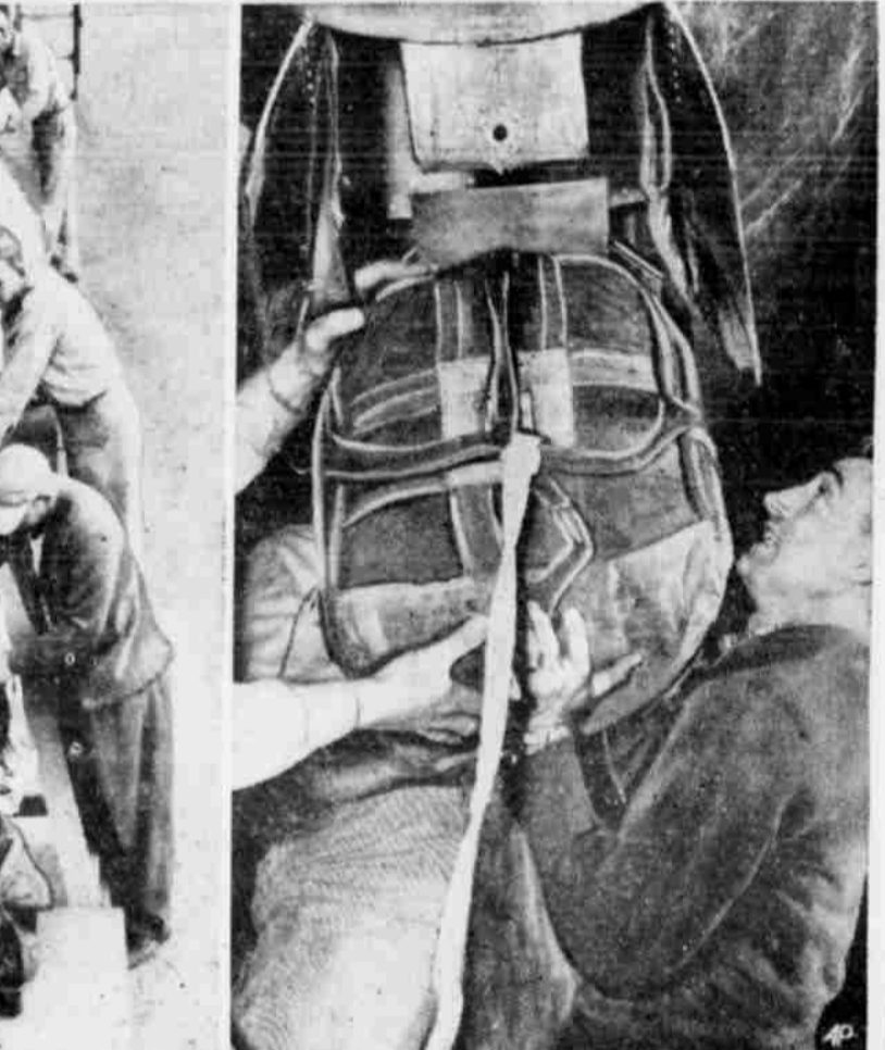
the larger chute into the slipstream. READY FOR USE, the parachute is loaded into a special compartment under the big plane's tail. A cockpit handle pops it into use.
