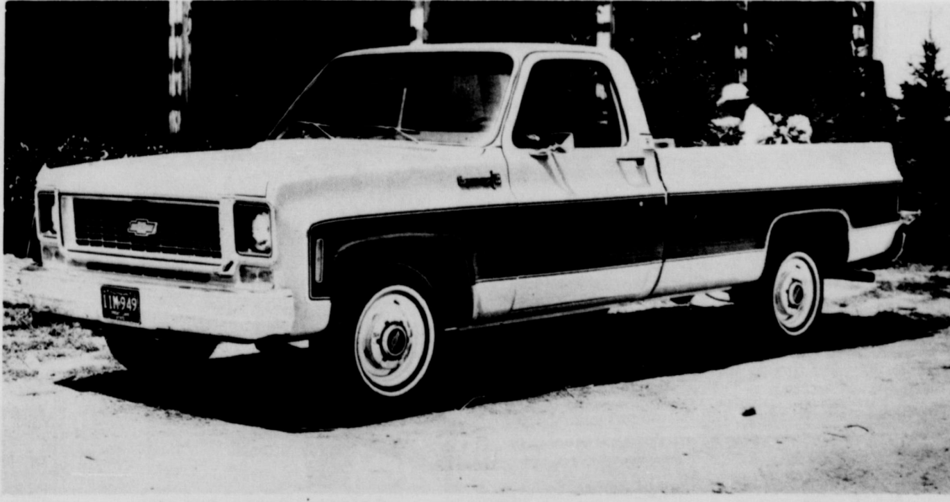
1973 CHEVROLET FLEETSIDE CHEYENNE SUPER PICKUP - Completely restyled and with extensive chassis redesign, the 1973 Chevrolet pickup line features many improvements in appearance, durability, and comfort for both commercial and personal transportation. Highlights are curved side windows, powered cab ventilation, new leaf-spring rear suspension, increased cooling capacity, a larger available engine, outside fuel tank, easier servicing, and highly styled interiors.
