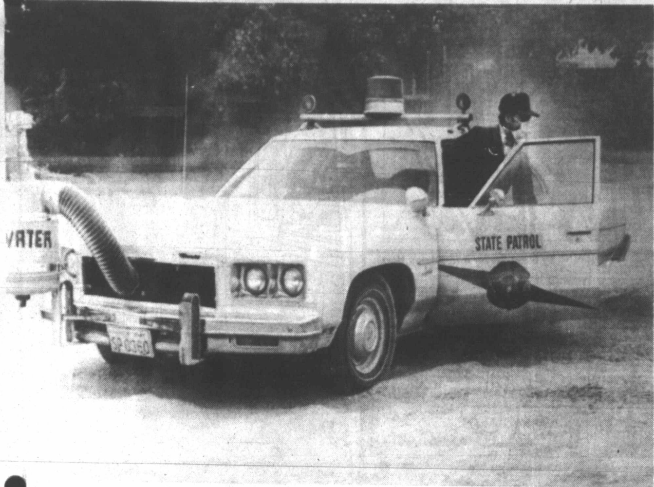
BEATING THE ASH PROBLEM with a fancy filter. Washington state troopers have donned gas masks and utilized truck air filters to stay on the job. The filters, marked "water" eliminate the clogging of engines by the tons of ash drifting and settling in the area. Scores of vehicles have been knocked out in the area due to ash build-up in cooling systems.
