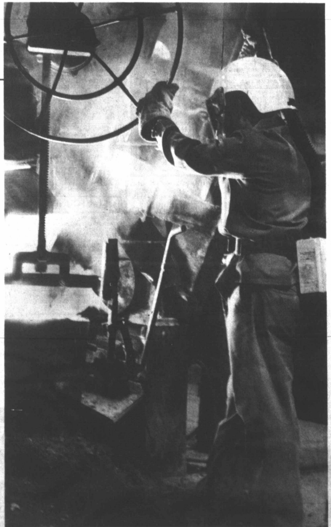
MOLTEN METERS. A foundry worker at Rockwell International's Uniontown, Pa., plant pours molten bronze from an electric furnace into a ladle. The molten bronze reaches a temperature of 2,400 degrees Fahrenheit and is used to make castings for the company's water meters. Rockwell is the leading manufacturer of water meters in the United States and has been making them for more than 100 years. The respirator the worker is wearing provides clean air to the face mask area.
