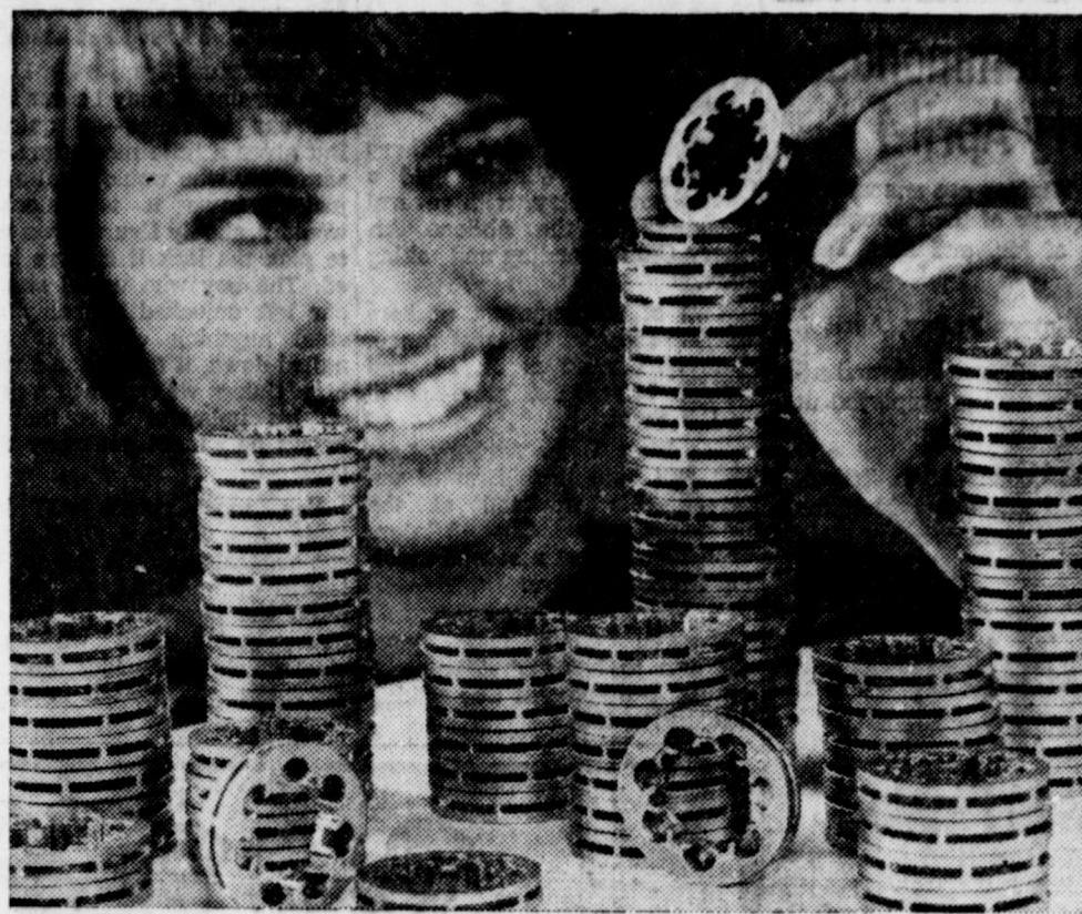
IN THE CHIPS , apparently, but Sonja Raftshol is not a big winner at Las Vegas. The disks she is stacking are actually sprockets for chain saws. The cutting chain whirls around the sprockets at more than 40 miles an hour when operating.
