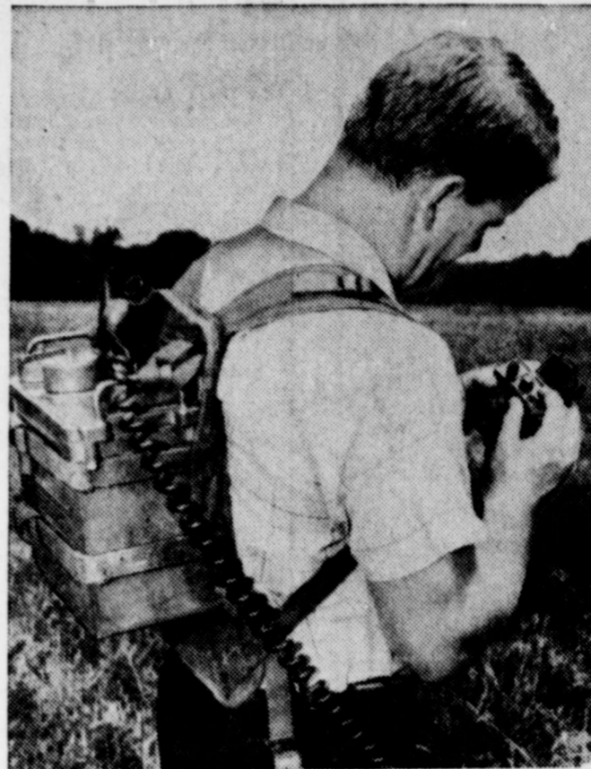
"WHERE AM I?" That question is answered instantly by small computer strapped to engineer's back. It automatically keeps track of every step he takes.
