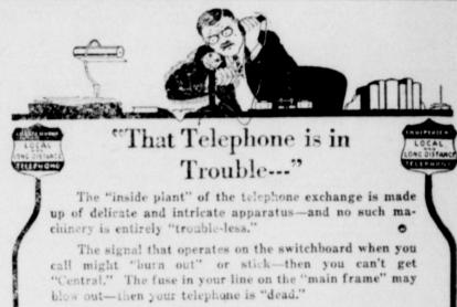
Switchboard cords are small flexible cables of many tiny wires; several of the little wires frequently snap from constant handling, then your connection "cuts off."
