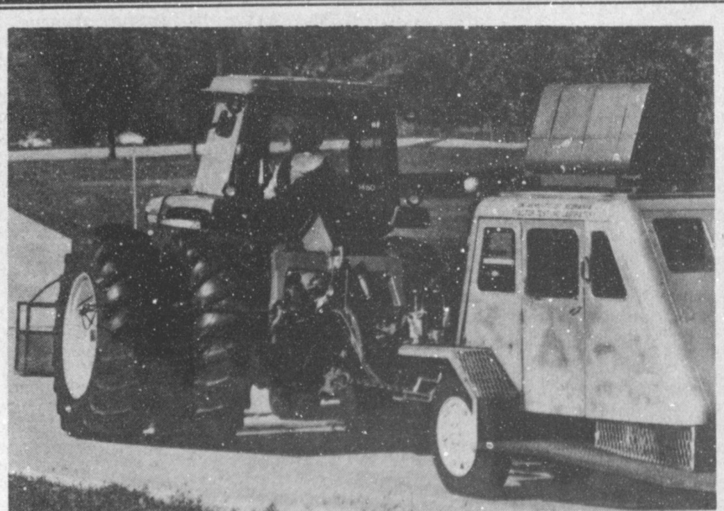
Official Nebraska test have been completed on all five of John Deere's new 100- to 190-hp tractors. According to Tuffy Dent of Dent-Rempe, the new 50 Series Tractors set records for PTO-measured fuel efficiency, drawbar pull and low sound levels. The 4850 shown above on the test track at Lincoln recorded 20,810 lb. of drawbar pull, the most ever for a 2-wheel-drive tractor.
