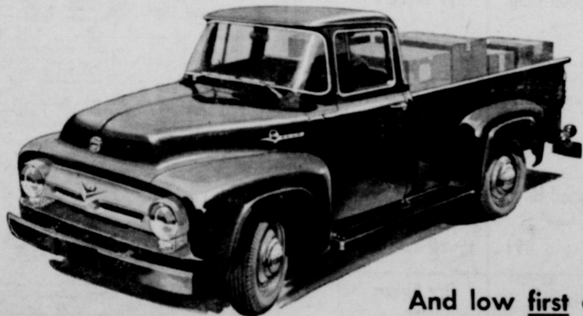
Ford's F-100 pickup with 8-ft. box is the biggest in the half-ton field—up to 19 cu. ft. more loadspace than the others. Regular 5 1/2-ft. box with a full 45 cu. ft. capacity also available.
