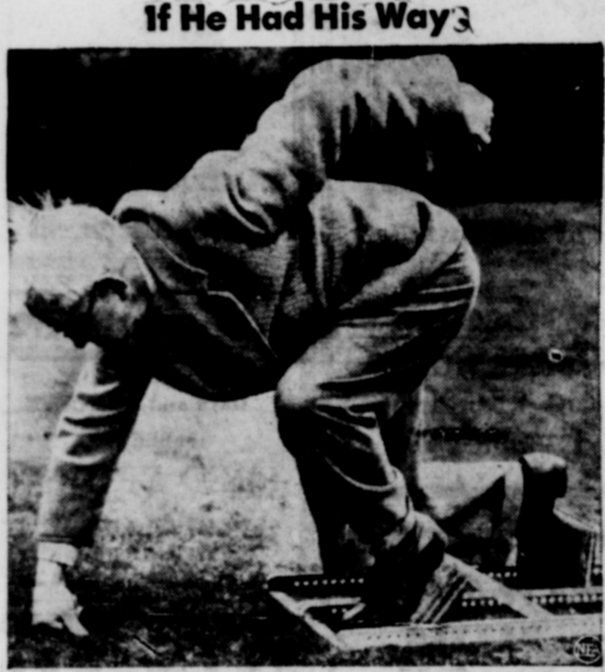
H. Hottenburg of London demonstrates the starting block he invented and his proposed starting style to help athletes in the Olympic Games this summer. The blocks can be moved backward or forward and be set at any required angle.
