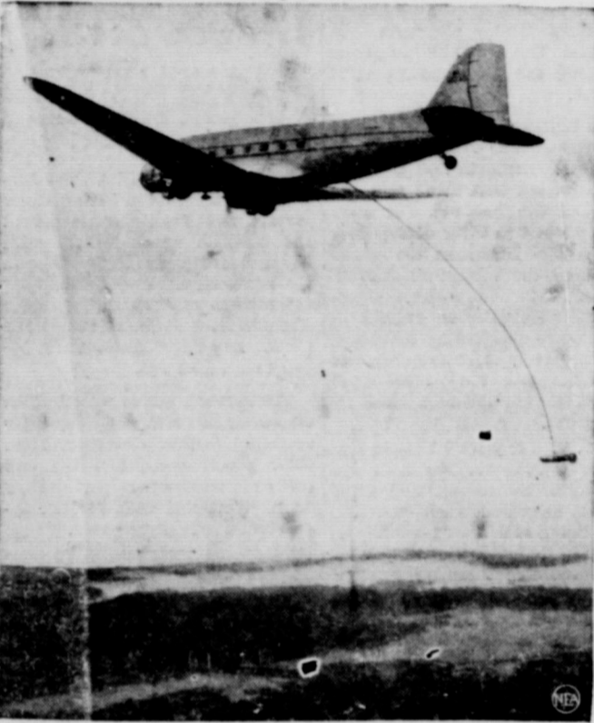
This airplane is prospecting for oil, using a newly developed airborne magnetometer. The instrument, which the plane trails as it demonstrates over Westchester Airport, N. Y., measures varying intensities of the earth's magnetic field. These are recorded in the plane, and data, which would take decades to gather on the ground, is quickly mapped.
