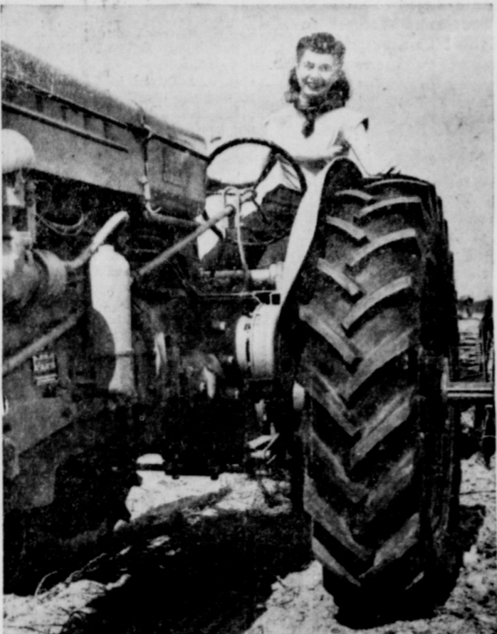
Something new in farm styling is proudly displayed by farmerette Bernice Davis as she enjoys a smooth ride on the new 1950 model curved bar, open-center tractor tires developed by The Firestone Tire and Rubber Company. Each traction bar is curved and tapered scientifically to improve its ground-gripping action upon biting into the soil and its self-cleaning action as it emerges from the soil. The new Firestone open-center farm tire is being offered in a complete range of tractor tire sizes to complement the traction center tractor tire line. This makes Firestone the first in the industry to offer farmers a complete line of tractor tires in several tread designs.
