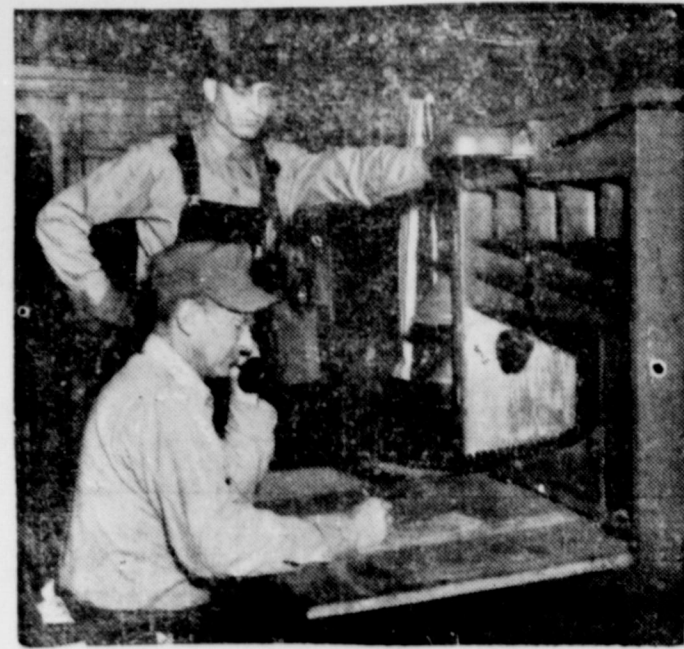
Texas & Pacific freight conductor W. F. Haworth, Sr., (seated) uses train radio 'phone in T&P caboose 2314 to contact engineer in cab 92 cars ahead, while rear brakeman H. F. Cooper stands by with walkie-talkie slung over his left shoulder.
