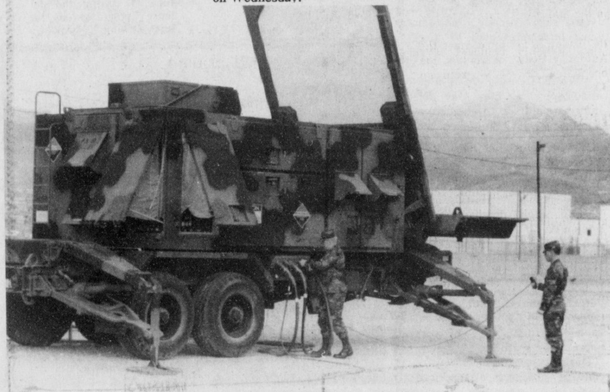
PREPARING A CONTROL CENTER--Sergeants attach electrical cables to a radar and engagement control center during training at Fort Bliss. The center, which is part of the Patriot system, uses its elevated radar screen to detect incoming aircraft and missiles. (U.S. Army photos by John A. Bohmer)
