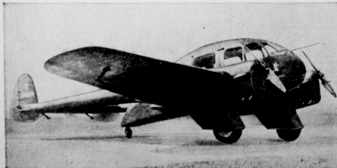
This queer-looking but speedy craft is the "Crusader," newly-built plane which could get you to Europe in 12 hours, if you so wished. The craft, designed by Thomas M. Shelton, will travel at a height of 26,000 feet and will make 300 miles an hour at cruising speed. The plane will make a Miami-Chicago hop shortly.
