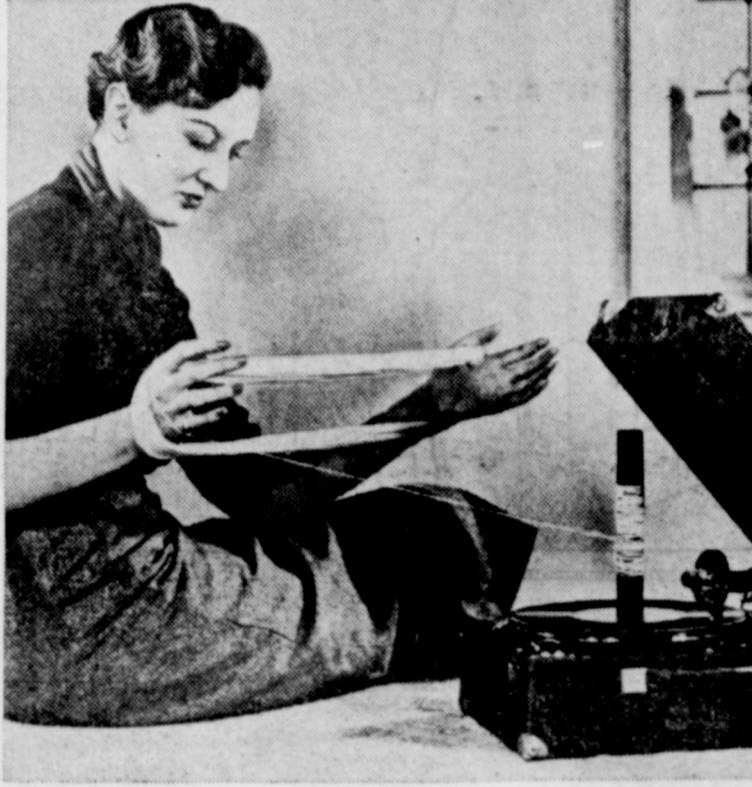
This young woman in England puts her gramophone to work spinning wool while she sits and enjoys the music. The wooden spool is pressed onto the centering post over the record.
