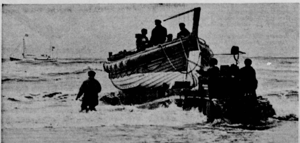
A new method of launching coast guard boats into surf is demonstrated on the coast of Holland. The equipment includes a tractor with caterpillar drive and a special truck for the boat.
